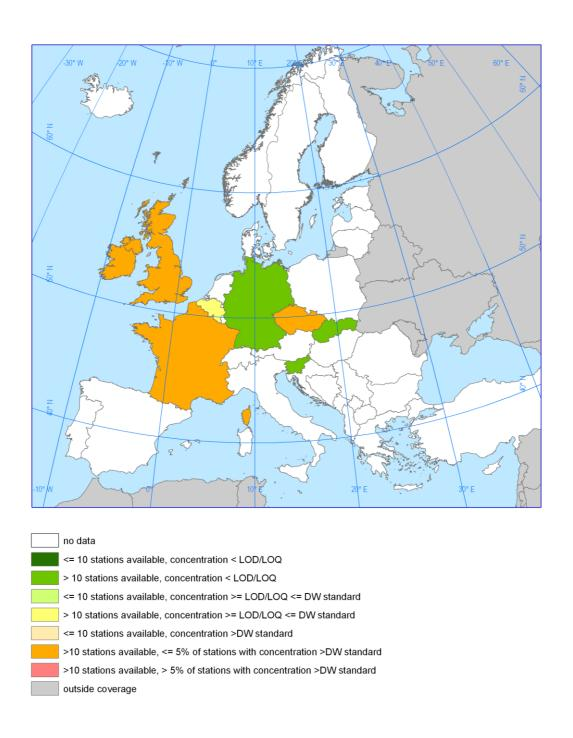
Figure 4.1.2.24a Long-term indicator (mean concentration, number of sites within indicator class) for mecoprop (MCPP) in groundwater
