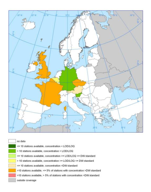
Figure 4.1.2.23a Long-term indicator (mean concentration, number of sites within indicator class) for MCPA in groundwater
