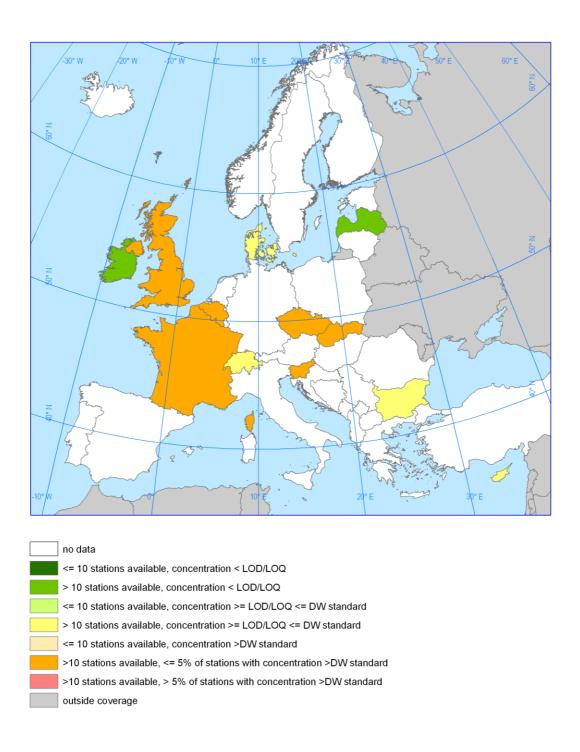
Figure 4.1.2.2a Long-term indicator (mean concentration, number of sites within indicator class) for 1,1,2-trichloroethene in groundwater
