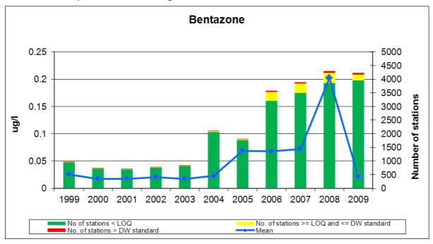
Figure 4.1.2.8b Indicator for bentazone in groundwater in 2008–2009 (number of stations per country shown in parenthesis)
